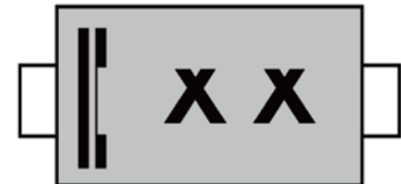
Bar = cathode marking XX = date code
